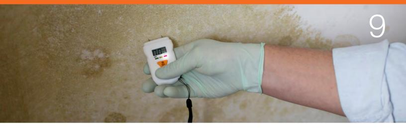
Rising damp, this type of damp and mould build up is usually a result of a long standard problem that has built up over many months or years, rising damp is primarily caused by the capillary action of water, which allows moisture from the ground to travel upwards through porous building materials like brick, joists and mortar. This occurs when a property lacks a proper damp-proof course (DPC) or if the existing DPC is damaged or bridged. External factors like decking or raised
